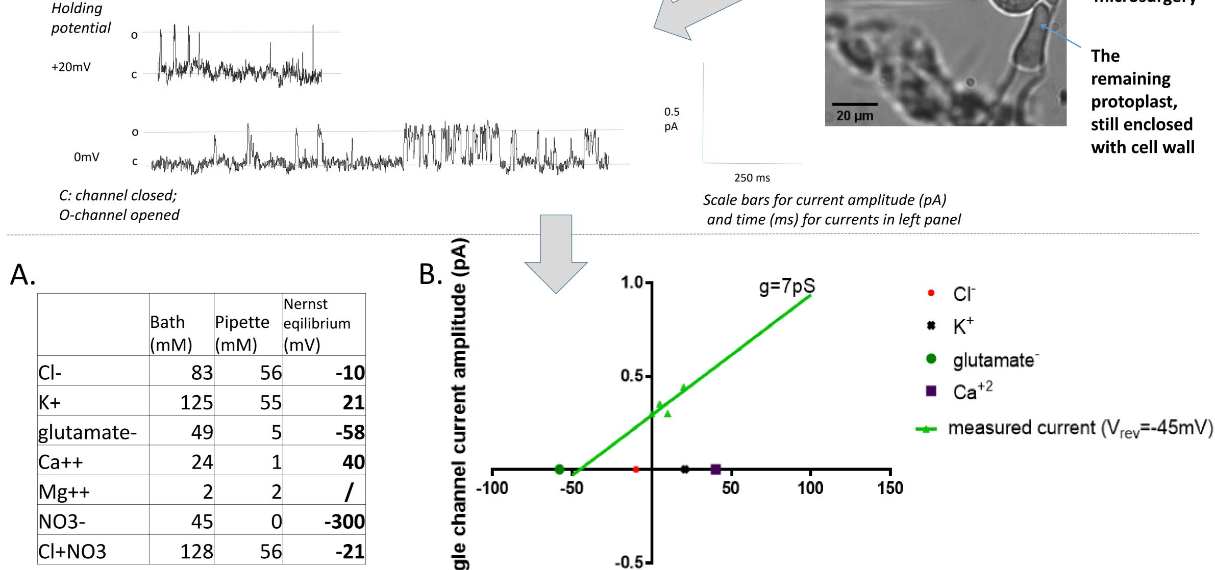
The example of the I/V graph constructed from single channel current amplitudes at several membrane potentials.
